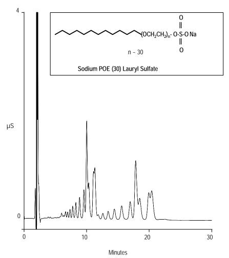
Figure 7 Analysis of POE(30) Lauryl Sulfate with Suppressed Conductivity Detection
