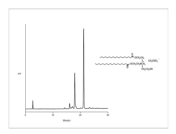
Figure 20 Analysis of Surfactants in a Fabric Softener
