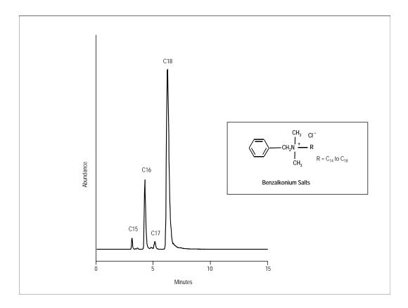
Figure 10 Analysis of Benzalkonium Salts with LC-ESI-MS Detection
