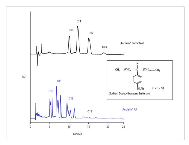
Figure 5 Separation of Linear Alkylbenzene Sulfonates
